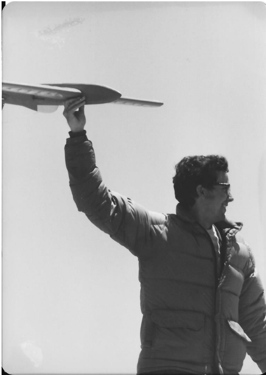
Sometimes Ken would launch the profile gliders upside down – it didn't matter because they came with a symmetrical airfoil. So long as the pilot was on the elevator quickly, it was quite fun. The airplane is a Goldberg Cosmic Wind.
